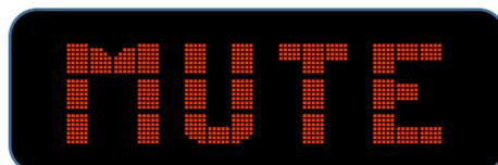
When the **MUTE** key is pressed, the *ZeroUno* DAC is muted and the display *never* switches back to the standard size view until the MUTE key is pressed again.
