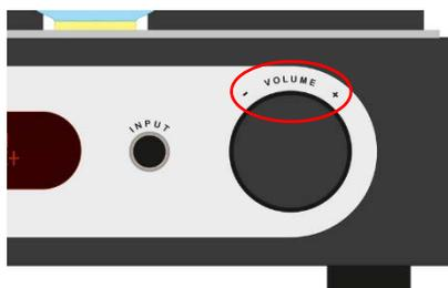
If no button is pressed or the right knob is not turned within 10 seconds, the *ZeroUno* DAC automatically stores the values shown at the display and switches back to the PLAY/MUTE mode.
