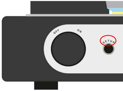
To **RESTORE** the factory setup, the SETUP button at the front panel of the *ZeroUno* DAC must hold for at least 10 seconds.
