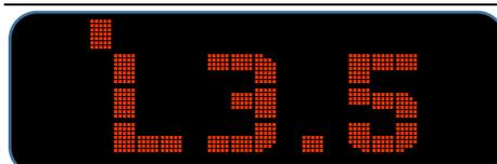
When the **BALANCE** keys are pressed, the balance changes in 0.5dB steps. Range is LEFT -5.0dB to RIGHT +5.0dB.
