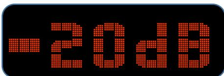
When the **VOLUME** keys are pressed, the attenuation changes with steps of 1.0dB. Range is -60dB to 0dB.
